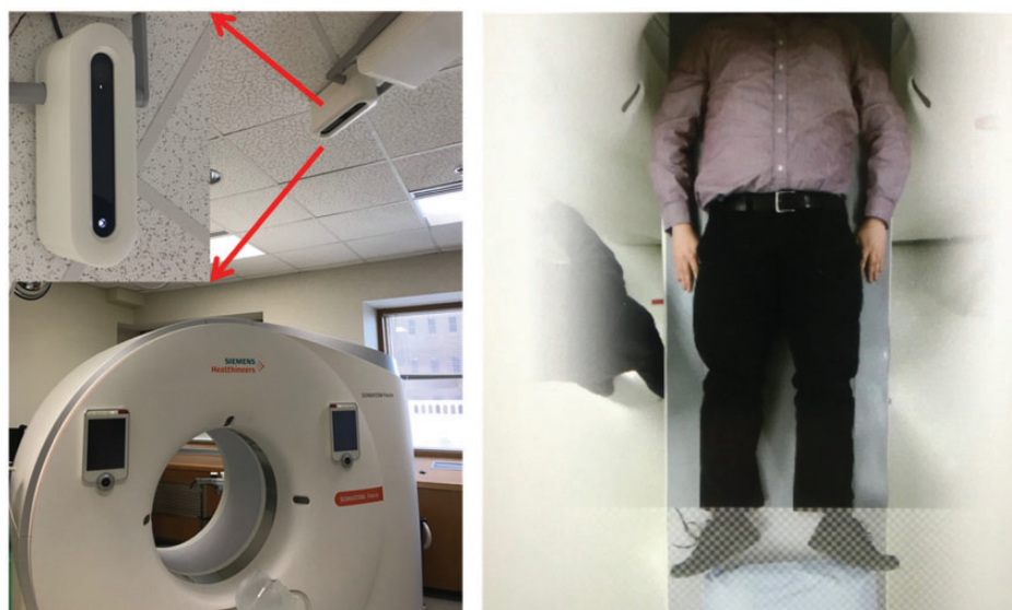
Fig. 4. The three-dimensional camera and its location above the patient table (left). Optical image and three-dimensional depth map of the patient acquired using the overhead camera (right).
